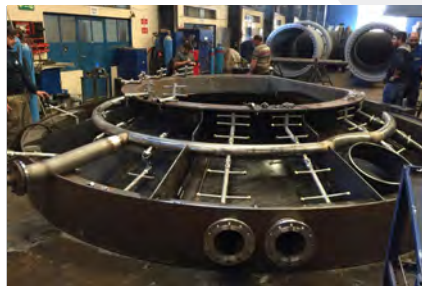
Open roof at BSE workshop displaying the collector ring and cooling elements
