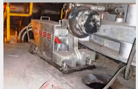
Flap mechanism device installed on the EBT panel for automatic opening / closing of the tapping access hole
