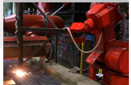
... realised by different flame modes for preheating and actual cutting process
