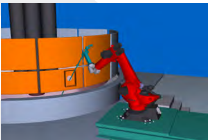
MultiROB with TempSamp function going through an opening in the EAF sidewall (Click picture to download simulation)
