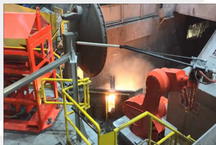
Automatic sample taking at ladle station with cartridge rack and tool exchanger (Click picture to download movie)
