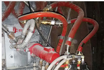
Tilttable VLB panel complete with hydraulic cylinder and hoses
