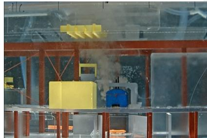
Fluid Dynamic Model of Stomana meltshop with simulated emissions from EAF
