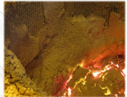
Skull formation at cold spots before installation ...
