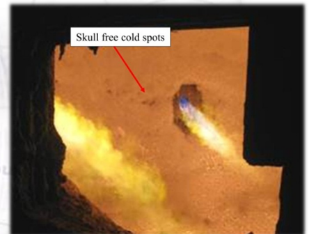
... and skull free cold spots after installation
