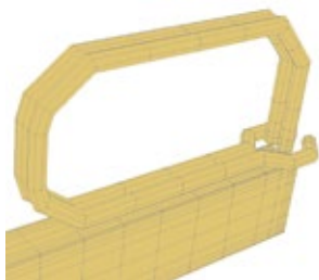
Symmetrising loop on centre electrode arm for optimum symmetry of reactances
