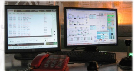
Touch screen at the operator pulpit for entering of a specific delay code by Jianbang operators
