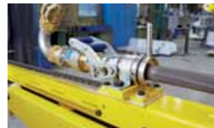
Snap-on coupling for fast and easy lance exchange
