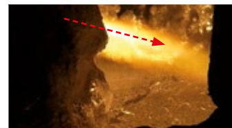
Flat angle of VLB for efficient meltdown of input material
