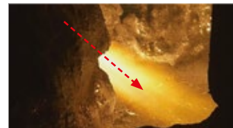
Steep angle of VLB for efficient injection of oxygen
