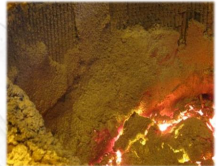
Skull formation at cold spots before installation ...
